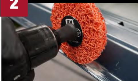
Remove seam sealer using the **QLock Strip It Wheel**.
